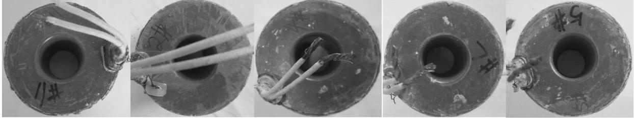
Fig.12 Coil assemblies after 7 d of heat exposure at 310 °C
