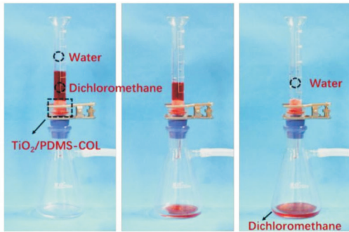
Fig.6 Continuous oil- water separation experiment under external drive
