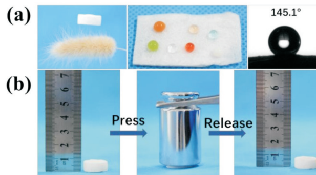
Fig.4 (a) Morphology and hydrophobicity of \text{TiO}_2/\text{PDMS-COL} sponge; (b) compression performance of \text{TiO}_2/\text{PDMS-COL} sponge
