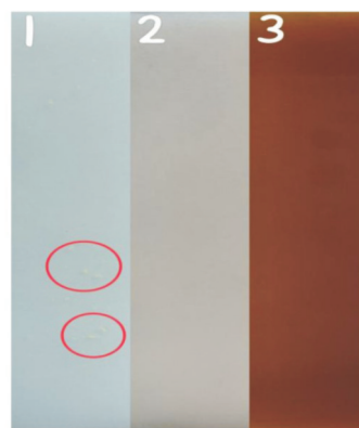
Fig. 6 Dispersion of composite particles in WEP emulsion (1): g-C 3 N 4 ; (2): g-C 3 N 4 @Fe 2 O 3 ; (3): g-C 3 N 4 @Fe 2 O 3 @CAQDs
