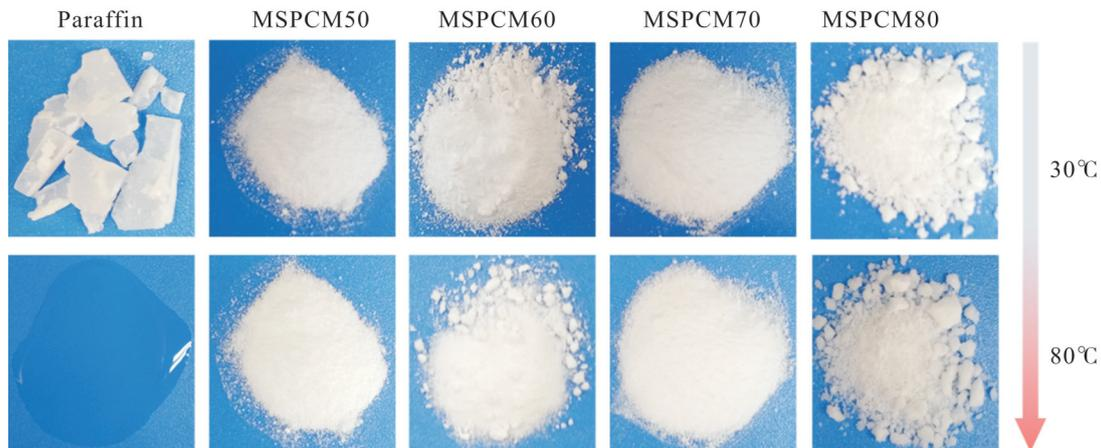
Fig. 9 Leakage testing of paraffin and MSPCMs
