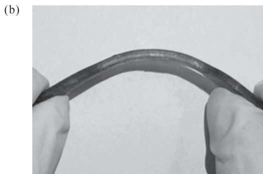
Fig. 8 (a) Bending stress-strain curves of PDCPD with different dosages of catalyst; (b) schematic diagram of PDCPD spline bending
