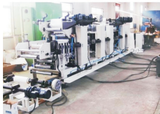
Fig. 7 Equipment for continuous fiber hot-melt prepreg
