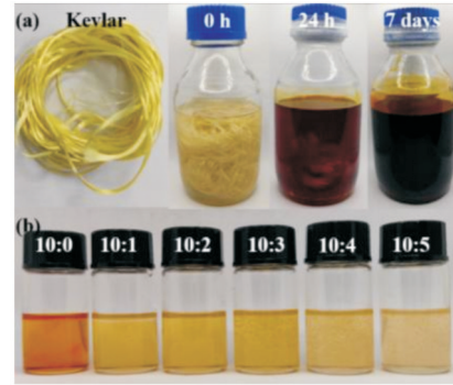
Fig.1 (a) Dissolution process of Kevlar fiber; (b) ANF solution after adding water
