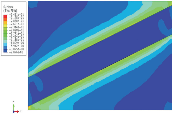
Fig.6 Local stress distribution in the initial loading phase
